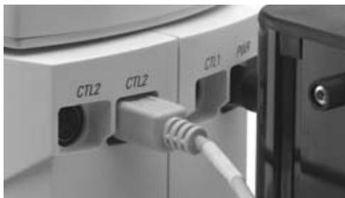
**Fig. 6** Rear side of Leica MZ16 FA with connections to power supply, motorized focus, manual controls, footswitch, PC
