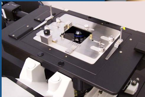
Applied Precision's patented Flexure Stage
